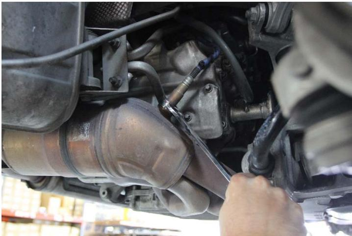
3. Using a 13mm socket, remove the (3) flange nuts from the studs.
