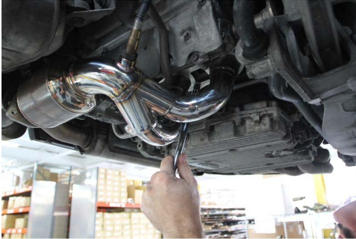
11. Re-position muffler bracket and insert/thread supplied 13mm hardware.
