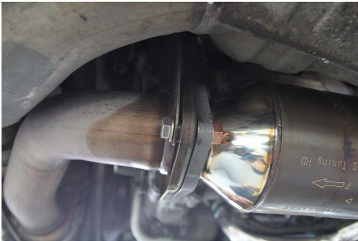
12. Tighten the (9) flange bolts using an E-12 inverted Torx (or 10mm socket). *Use hand tools only!*
