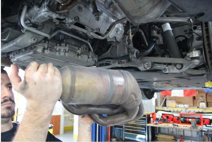
8. Hang Fabspeed header and re-thread the rear O2 sensor and tighten with a 22mm wrench.
