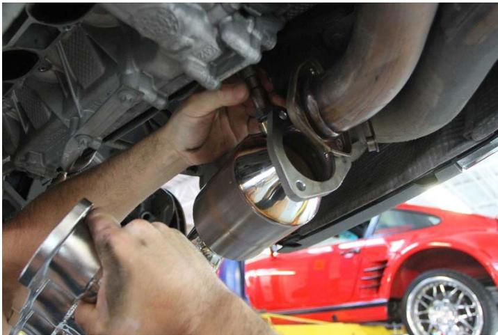
9. Thread the front O2 sensor and tighten with 22mm wrench.
