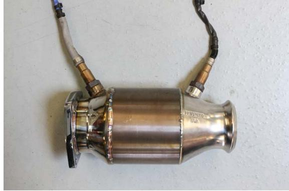
17. Hang the Fabspeed Sport Cats on the turbo studs and tighten the (4) flange nuts.
