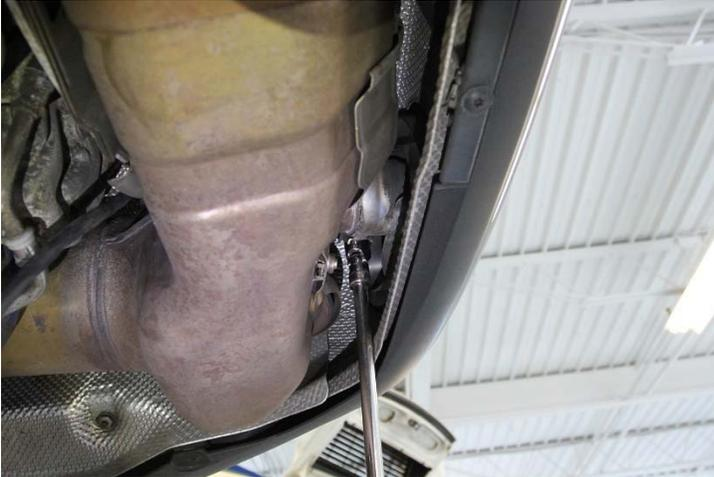
14. Using a 6mm Allen bit, loosen and remove the (2) band straps securing the factory muffler.
