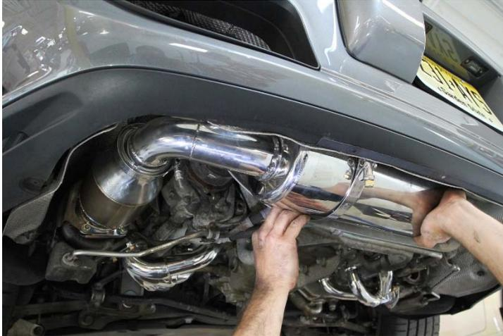
20. Using an 11mm deep socket, tighten the v-band clamp.
