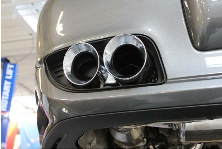
23. Align tips to desired position and tighten the clamps in the back with a 13mm socket.
