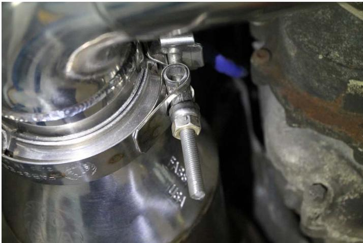
21. Using a 13mm socket, tighten the band clamp.
