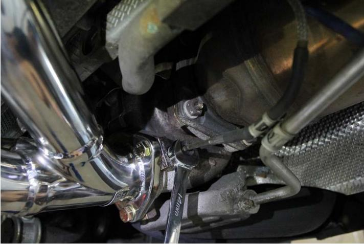
11. Using a 13mm wrench, remove the (4) nuts securing the catalytic converter to the turbo.
