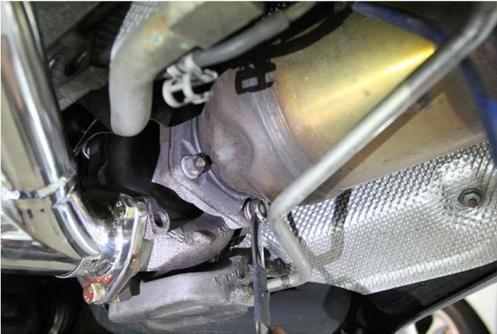
12. Using an 8mm wrench, remove the bolt securing the outside of the turbo heat shield.
