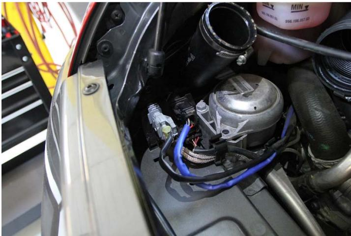
9. Raise the vehicle and fish the O2 sensor wires down through the engine so that they are freely hanging below the vehicle.
