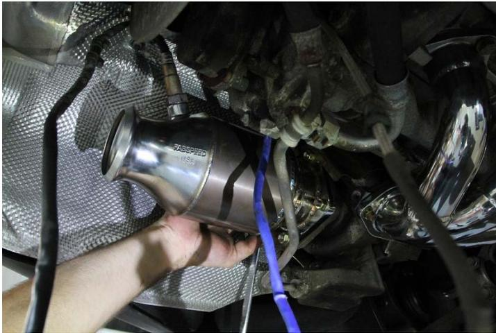
18. Re-insert and tighten the bolt securing the turbo heat shield on either side of the car.
