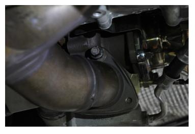
16. Using an E12 inverted Torx or a 10m socket, remove the (9) bolts securing the main header flange to the engine block and remove the header from the vehicle.
