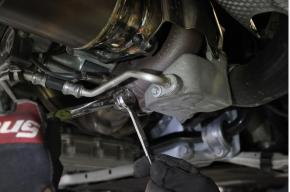
14. Back the studs out of the header using a 13mm wrench on the bottom nut, closest to the flange.
