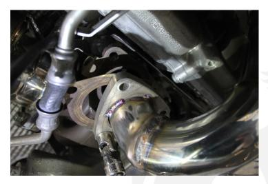
20. Using an E12 Torx or a 10mm socket, insert the remaining (8) header flange bolts. Do not tighten each one until they are all in place.
