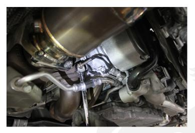
8. Using a 12mm wrench, remove the remaining nut from the header/turbo flange.
