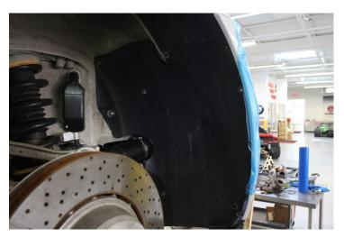
4. Remove fender liner from wheel well.
