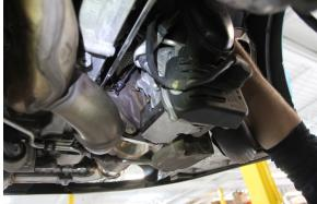
Using a 12mm socket, remove the exposed header/turbo flange nut.
