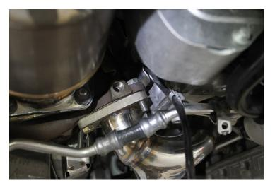
22. Tighten all nuts and bolts, moving from the center outwards on the header flange.
