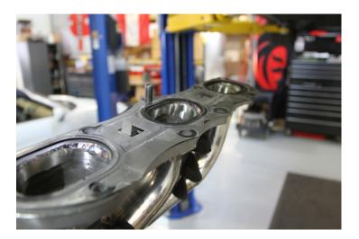
18. Position left side header on engine block and finger tighten the header bolt to hold the header in place.
