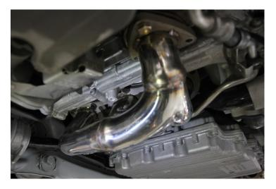
19. Insert the remaining triangle gasket and loosely thread the supplied 13mm bottom bolt into the turbo flange.
