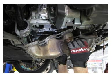
12. Using a 12mm wrench, remove the (2) nuts from the bottom of the header/turbo flange on the right side header.
