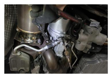
9. Using a 8mm socket, remove the oil line bracket bolt so that the oil line can be moved slightly during the removal of the header.
