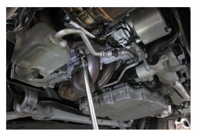
7. Using a 14mm wrench, remove the EGT sensor.
