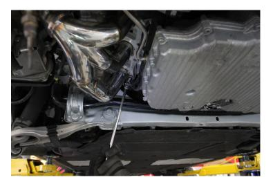
21. Insert the (2) supplied 13mm bolts/washer down through the turbo flange and thread on the supplied 13mm nuts and washers.
