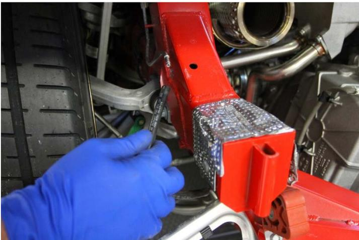
3. Using a 10mm socket, remove the bolts securing the factory vacuum lines from either side of the vehicle. Unclips the lines from the inside of the support brackets, and remove the lines.
