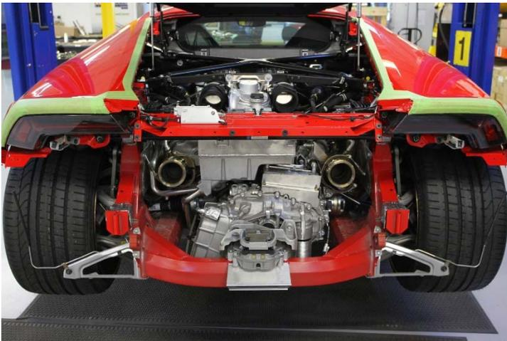
2. Remove the rubber vacuum hose section from either side of the vehicle.
