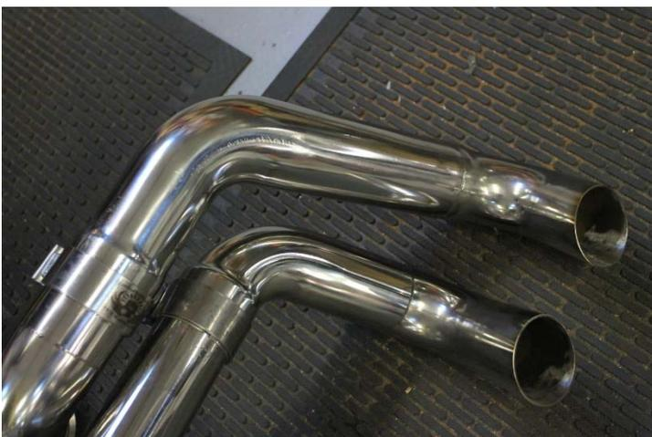
6. Using the supplied 13mm bolts and nuts, install the mounting brackets on the inside of the Fabspeed X-Pipe as pictured.
