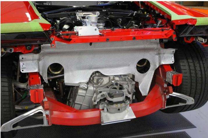
5. Install tail pipe sections on to the Fabspeed X-Pipe. Be sure to face the clamp bolts towards the front of the vehicle to allow access from the wheel well. Do not fully tighten at this time to allow for final adjustments.
