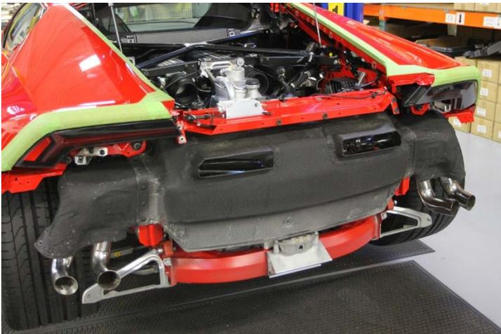
11. **NOTE:** Before re-installing fender liners, position tail pipes and tighten the 15mm Accu-seal clamps to secure in position.
