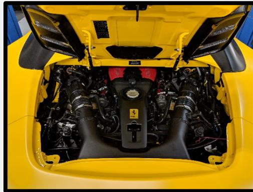
9. Then remove the maf housings and couplers to gain access to the cat pipe mounts.
