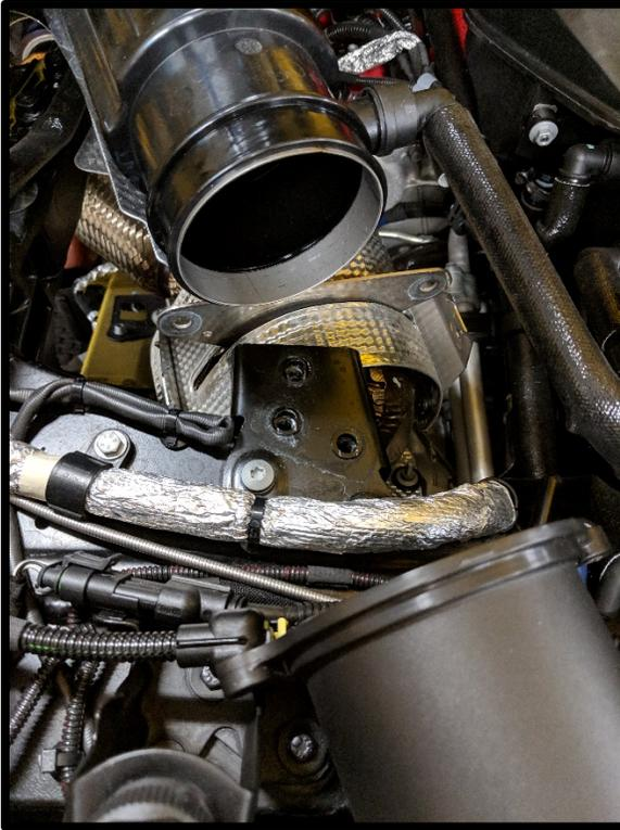
11. Now remove the cat pipes by twisting them back and forth and pulling them out of the exhaust. A little penetrating lube helps here.
