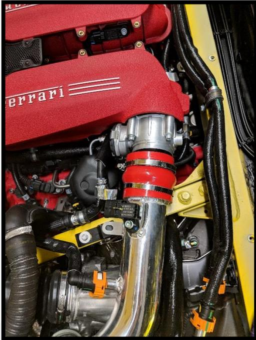
14. Before tightening the hose clamps, make sure the charge pipe is seated in the hoses at both ends sufficiently. Once satisfied with the fitment, tighten clamps, reconnect the map sensor, EVAP hose and mounting nut.
