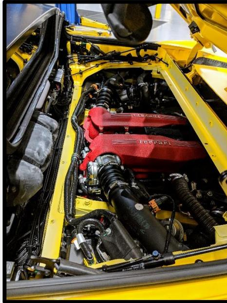
8. Once you gain access to the factory intake charge pipes, start by disconnecting the map sensor plug by sliding the locking clip outward and gently pull off the connector. Repeat for the other side.
