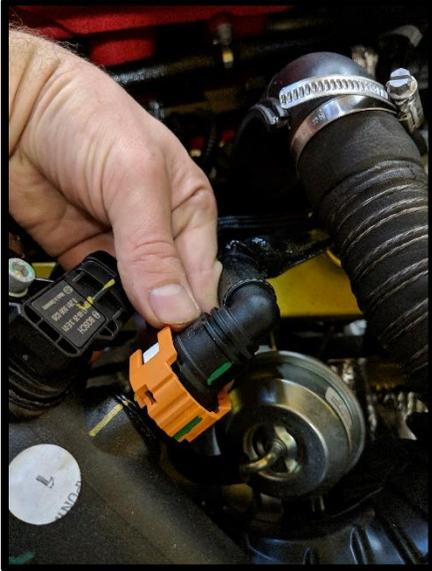
10. Next unbolt, the 10mm mounting nut on either side. You can now loosen the band clamp at the throttle bodies and remove each pipe.
