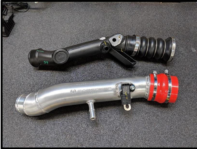
12. You can now install the Fabspeed Intake Charge Pipes by first inserting them on the intercooler outlets. Some lubricant such as wd40 helps here.
