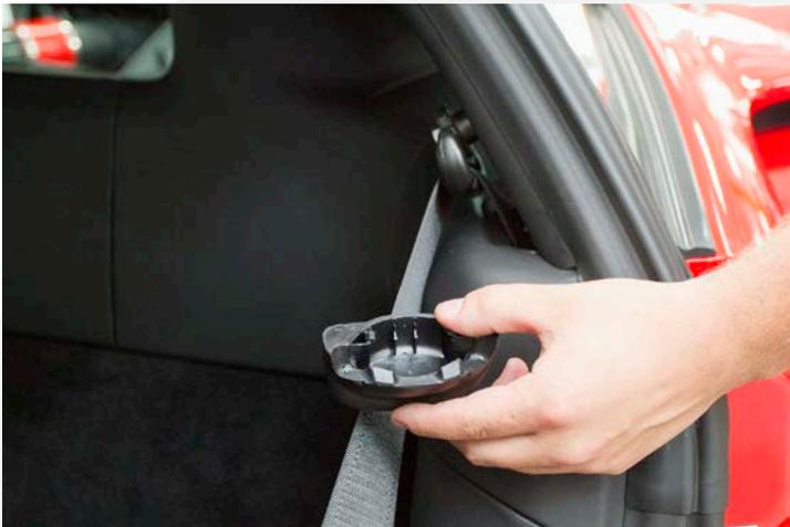
3. Using a 17mm socket, remove the upper seatbelt mounting bolts.
