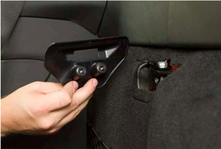
8. Using a 13mm socket, remove the top mounting bolt.
