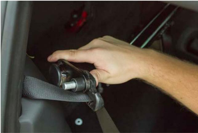
11. Thread the bolt back into the side pillar and finger tighten. Do not fully tighten at this point.
