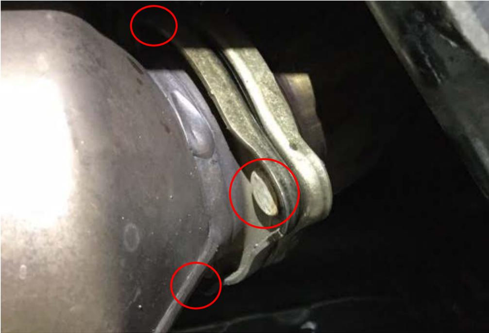
2. Loosen (*do not remove*) the two (2) 13mm Torca clamp (side clamp) bolts at the rear of either factory secondary catalytic converter, and slide the clamps back.
