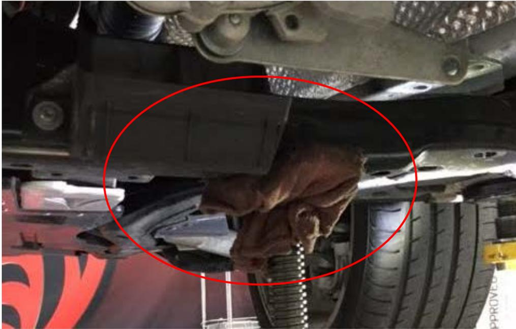
6. *(Optional)* Loosen two (2) 16mm bolts on either side of the transfer case crossmember. Depending on year and model, you may not need to remove the brace, but rather loosen it just enough to maneuver out the factory secondary catalytic converters.
