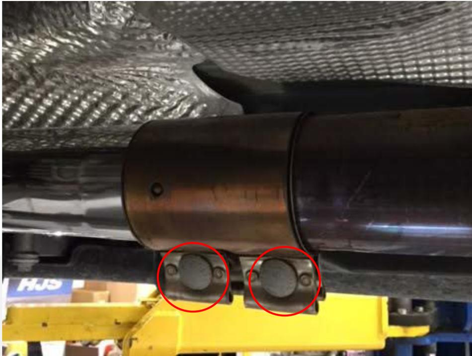
11. Hand tighten center mounting bracket bolts using factory 13mm hardware.
