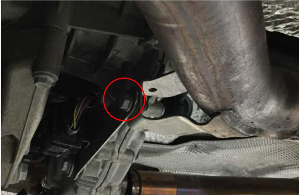
4. Carefully maneuver secondary catalytic converters out of place by sliding them towards the front of the vehicle. *(Note: Depending on year and model, it may be necessary to loosen transfer case crossmember to remove catalytic converters).*
