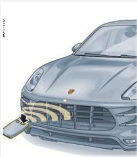
4. Stand in front of the vehicle with the Fabspeed key FOB approximately 12" away from the center of the radiator grille.
