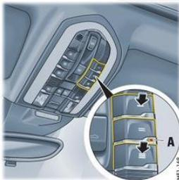
3. Decide which button on the overhead console that you want to teach to operate your exhaust valves to the **open** position. Press and hold the desired button until the indicator light flashes. You have 5 minutes to teach the button.
