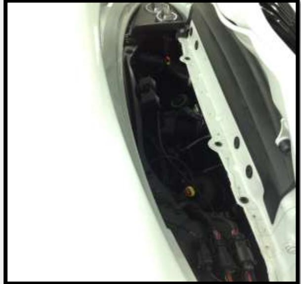
5. Remove spoiler base hardware. (x2) T30 bolts. Pushing forward on the very trailing edge releases the remaining clips. Spoiler base cover is now free. Lift up and tape to extended spoiler.
