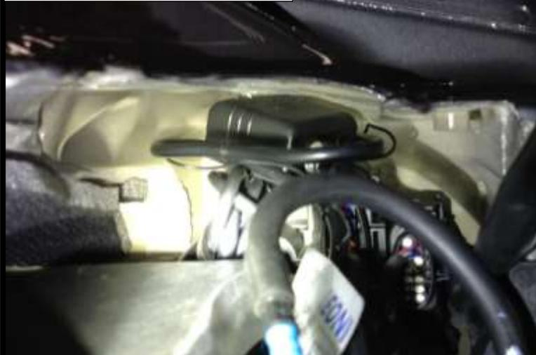
Upper right-hand corner of the engine compartment above the engine harness bulkhead connectors is a safe, dry location away from heat.
