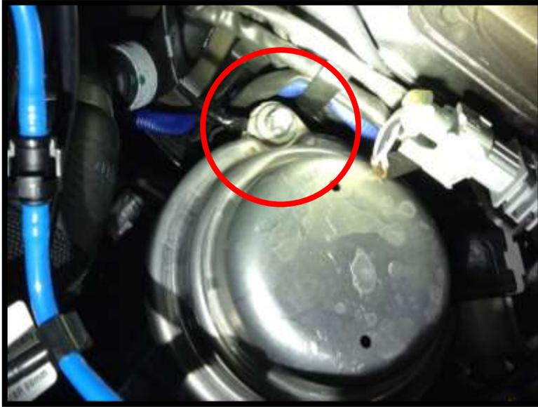
16. Suggested plumbing and wire routing for a clean install. Secure with zip ties away from heat, rain water, and moving parts. Be sure to not rub on a sharp edge that can chafe through and cause future problems.
