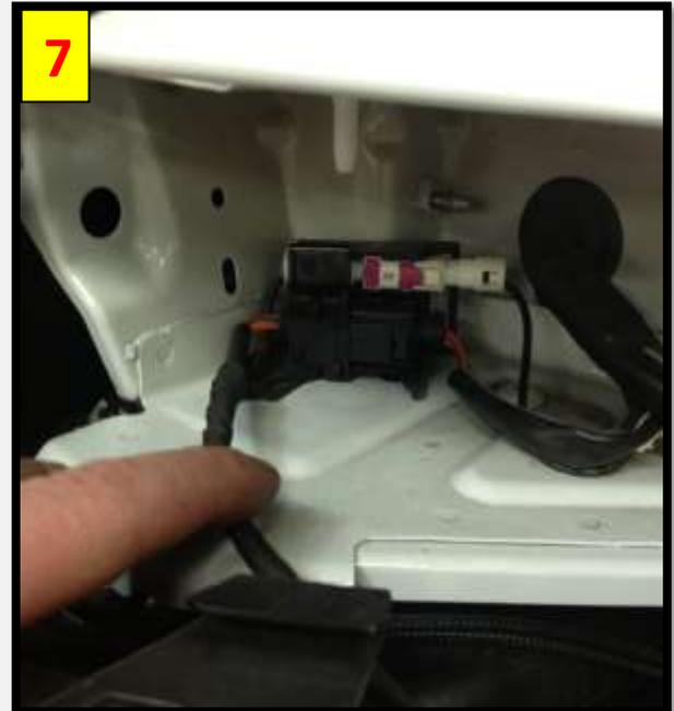
7. Disconnect the rear bumper harnesses. (x2) Behind right side taillamp. (x1) Behind left. Tip: taping them to the bumper cover makes reassembly easier and prevents missed connections.
