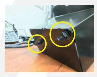
Slide the silicone coupler over the existing factory intake hose and tighten both hose clamps. Attach the vacuum line as shown.
