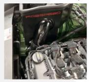
After lining up the bottom mounting bolts on the heat shield assembly with the factory silicone mount points, you will be able to drop in your new Fabspeed intake system.
