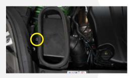
You will then need to detach the vacuum line from the stock intake tube as well as loosen the hose clamp using a slotted screwdriver. You will be provided new hose clamps.
