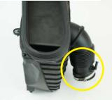
Insert your new Fabspeed intake pipe through the hole in the head shield assembly as shown.
