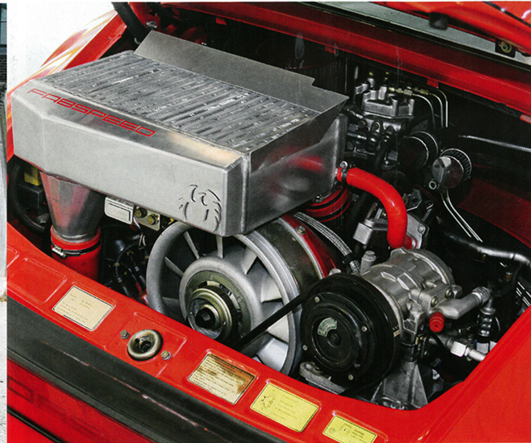
Clockwise from opposite: The 18-inch HRE three-piece modular wheels fill the Turbo fender flares nicely. That's a monster-sized Fabspeed intercooler! The 505 option sticker proves the car's pedigree. Fabspeed custom plumbing ensures zero leaks for maximum boost. A factory 930S bumper completes the visual package. That 1980s 911 interior is both classic and as comfortable as your favorite chair.
