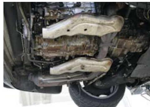
The original heat exchangers (above) ready to come off. Without an exhaust, you get a good look at the flat six engine
