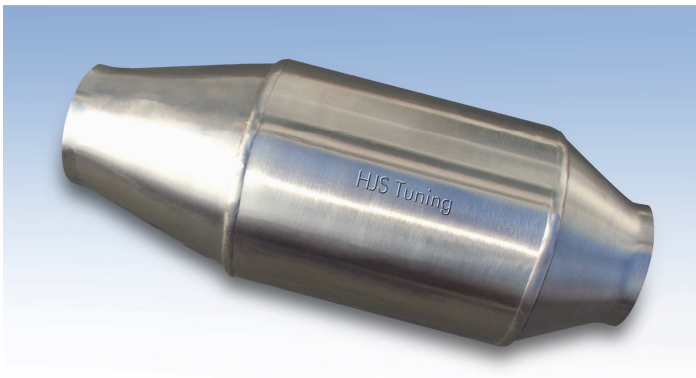
HJS - High Performance Converter with 200 cell metal matrix .
