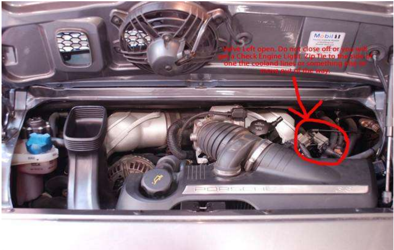
STEP 6: Lift the oil fill from the airbox.
